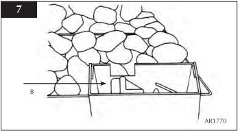
7.5 Ensure that the fibre glass window seal on the box is intact. Lower the glass window into the hooks on the box. Secure the window using four screws in the retaining bracket, Diagram 8.
